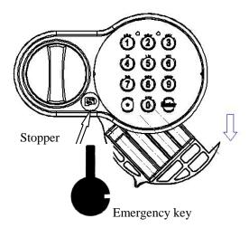
Attention! Set the emergency key in the horizontal position. The cut of the key should be on the right as shown in the picture.
